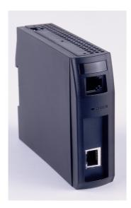
The MODBUS/TCP Bus Module is part of the MLC 9000+ DIN-Rail mounted multiple loop PID control system. The Bus Module is the supervisor in the MLC 9000+ system and manages the communication with up to 8 single or multiple Loop Modules and the MODBUS/TCP network. Systems larger than 32 loops can be built using multiple Bus Modules, within the limitations of your MODBUS/TCP system.
