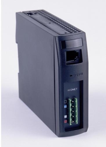
The DeviceNet Bus Module is part of the MLC 9000+ DIN-Rail mounted multiple loop PID control system. The Bus Module is the supervisor in the MLC 9000+ system and manages the communication with up to 8 single or multiple Loop Modules and the DeviceNet network. Systems larger than 32 loops can be built using multiple Bus Modules, within the limitations of your DeviceNet system.
