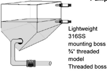
Many processes have batching and header tanks, and there is usually the need to control a pump to maintain levels between set points, keeping the process supply line going. These tanks are often manufactured from thin wall materials and cannot support the weight of heavy instrumentation.
