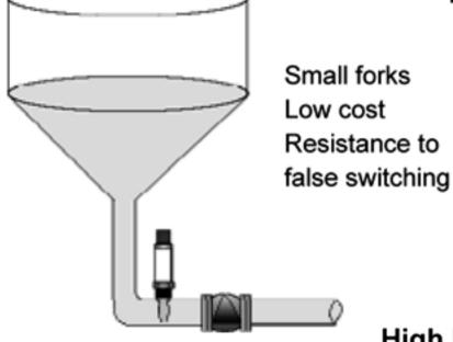
Pumps are not cheap. Damage a pump by running dry and the costs multiply, not least being equipment replacement and consequent downtime.
