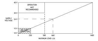
Max Output Load [(Vsupply -10)/21.5] KW, 250  $\Omega$
