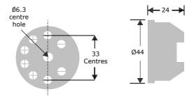
M4 Spring loaded fixing and screws (supplied)
