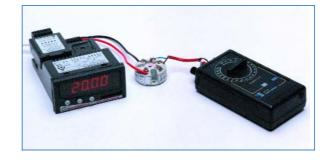
TYPICAL SET-UP The above picture shows SEM203TC, DM3420 Indicator, and Thermocouple simulator.
