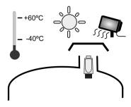
The transmitter must be installed in a location where it is protected from ultraviolet radiation, in order to prevent long term degradation of the plastics used in its construction e.g. shrouded from direct sunlight.
