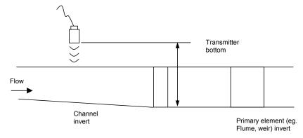
In addition to the above, when setting the bottom reference on a 'V' notch weir it is important that the true invert of the weir is taken and not the meniscus liquid level, which may be 3 to 4mm above the true invert.
