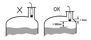
If the transmitter is mounted in a stand-off or nozzle, it is always preferable that the transmitter face be at least 5mm proud of the stand-off such that it protrudes beyond the stand-off and into the tank.
