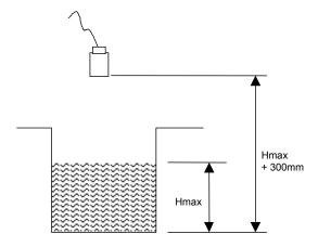
It is important to note that the bottom reference of the transmitter should be related to the centre of the invert of the primary device, NOT the distance to the channel bottom directly below the transmitter.
