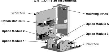
To access modules 1. A or B. first detach the PSU and CPU boards from the front by lifting first the upper, and then lower mounting struts. Gently separate the boards. Plug the required option modules into the correct connectors, as shown below.
