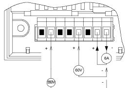
Connect only one input at any time to the indicator. Wherever possible connect the neutral side or circuit common to the input terminal.
