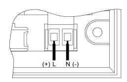
To minimise potential noise problems, power the indicator from the same power branch or phase as that at the signal source
