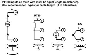
For cable length < 3 Metres no screen or twist pair required. Thermocouple inputs must use correct compensation cable.
